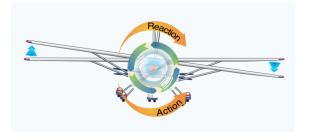
generally designed so that the left wing makes slightly more lift than the right wing (which also
