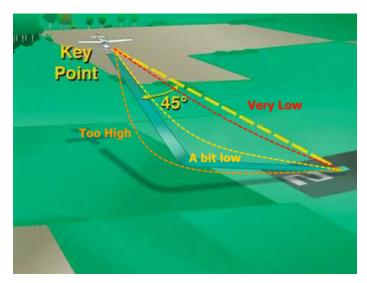
Airspeed - Flying at an airspeed faster than, or slower than, best glide speed will result in a shorter glide.
