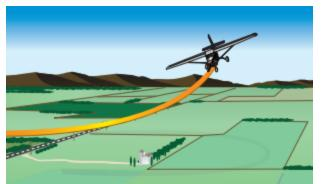
Spiral - In order to maintain positive load factors throughout, and to remain over a potential emergency landing area, an emergency descent is often flown as a steep, spiraling descent. In most cases, the objective is to rapidly descend to a suitable landing area where an emergency approach and landing can be executed. Therefore, a good point on the ground to spiral over is the 'downwind key position' for the eventual emergency landing location.
