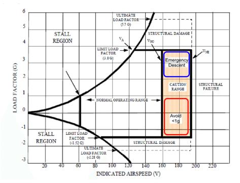
Entry - Generally, the proper entry for an emergency descent is to reduce power to idle, begin a 30-45 degree banked turn, and lower the pitch angle to accelerate to Vne or Vno, as appropriate.
