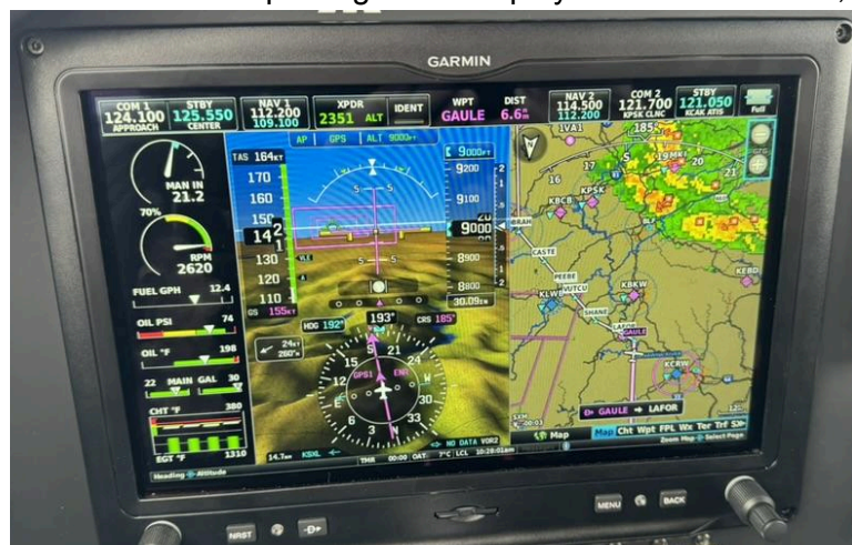
A Garmin G3X Touch displaying NEXRAD data in-flight.
