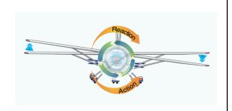
Spiraling Slipstream - As the airflow moves through the propeller and around the fuselage, wings, and control surfaces, it is spinning. The spinning propeller imparts a considerable spiraling motion to the slipstream, and because the vertical tail surface extends only above, and not below, the spiraling slipstream pushes the tail slightly right, leading to left yaw.
