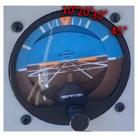
self-correcting instrument, and as the gyroscope *precesses* (is affected by friction), it makes small corrections to remain upright.
