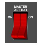
■ Shed electrical load - If electrical overload is the suspected cause, begin by turning off unnecessary electrical accessories or secondary radios.
